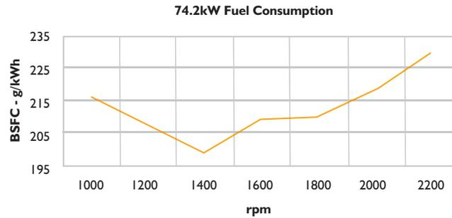
Fuel consumption with fuel at 40°C pump inlet, at full load.
